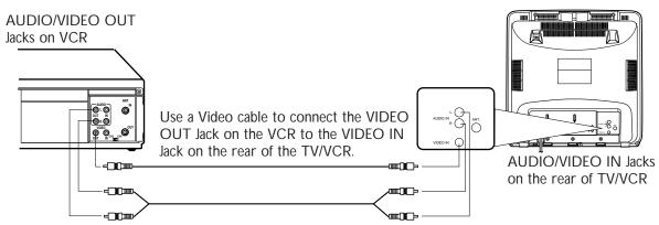
Use an Audio cable to connect the AUDIO OUT Jacks on the VCR to the AUDIO IN Jacks on the rear of the TV/VCR.
